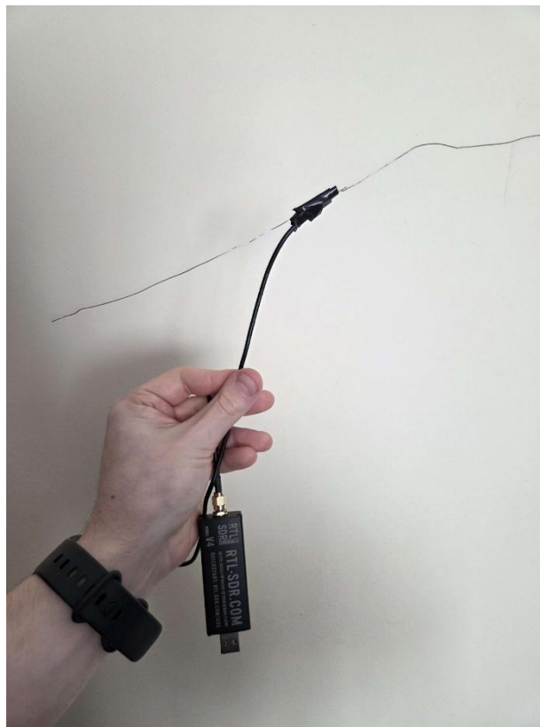
Figure 42: An RTL-SDR hooked up to a custom-made dipole antenna for real-time analysis of wireless communications.
