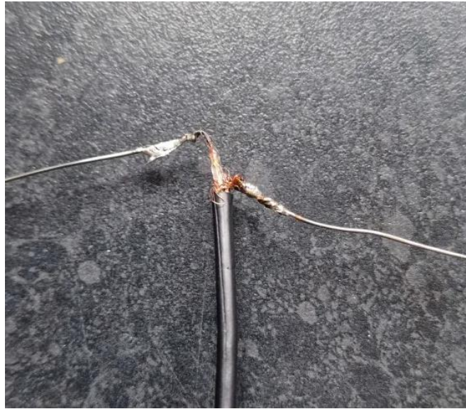
Figure 31: Soldered dipole antenna utilising coaxial cable and two 6.8" jumper wires to create a homemade dipole.
