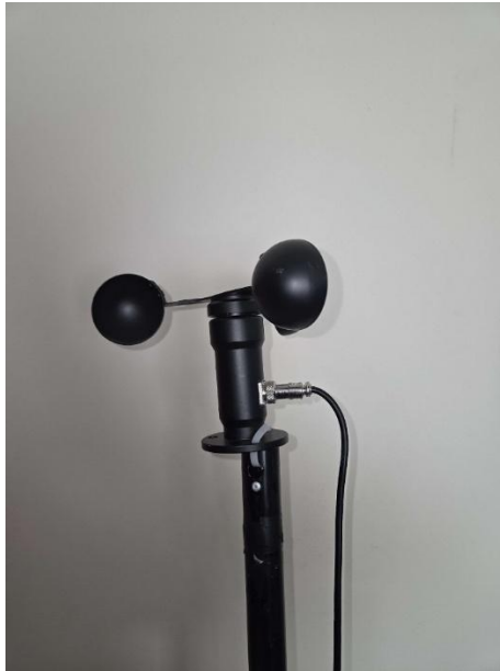
Figure 39: Replacement anemometer utilising an analogous transmission scheme.
