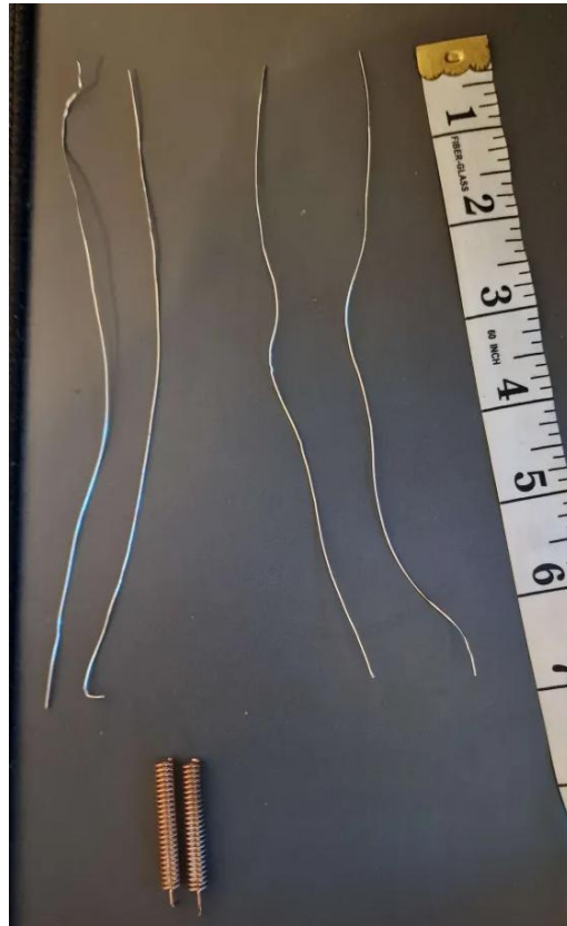
Figure 29: Two sets of ~6.8" wires used for the separate sides of the dipole antennas.
