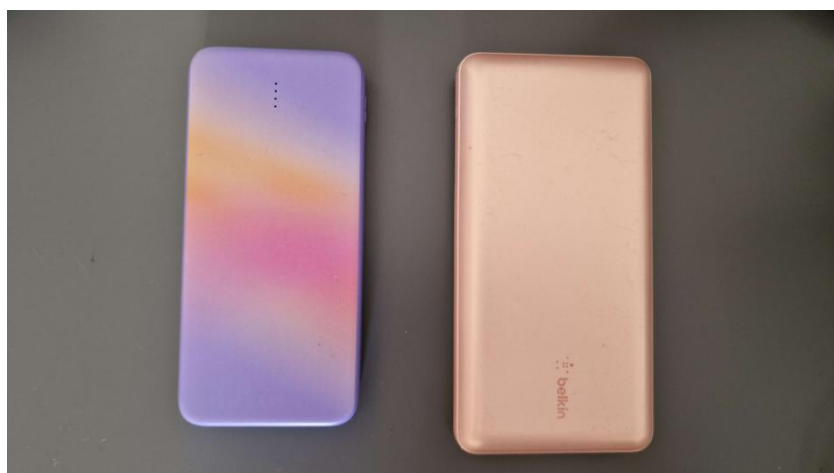
Figure 24: Acquired battery banks for off-grid operations, providing up to 227 hours at 10000mAh (left) and 454 hours at 20000mAh (right)
