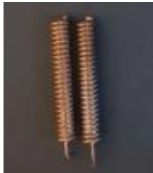
Figure 28: Two spring antennas for low distance communication tuned to 433mhz.
